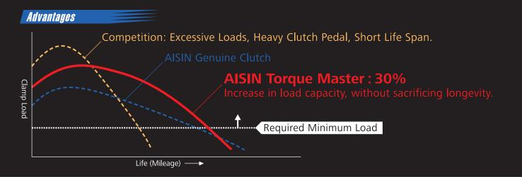
Excessive clamping loads cause heavy clutch pedal feeling, shorten the life of the clutch, and may cause damages to the clutch operating mechanism.
