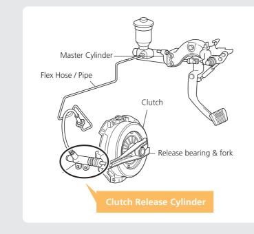
The clutch release cylinder (also known as the clutch slave cylinder) is the component that transfers hydraulic pressure, achieved through the clutch master cylinder, into a mechanical force to control the clutch fork. The force from the release cylinder engages and releases engine power to the transmission.
