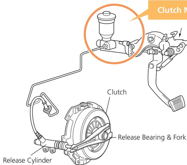
The clutch master cylinder is a device that transforms mechanical force into hydraulic pressure. As the driver presses the clutch pedal, the pedal lever applies force to the clutch master cylinder which transmits hydraulic pressure to the clutch release (slave) cylinder that disconnects engine power to the transmission.
