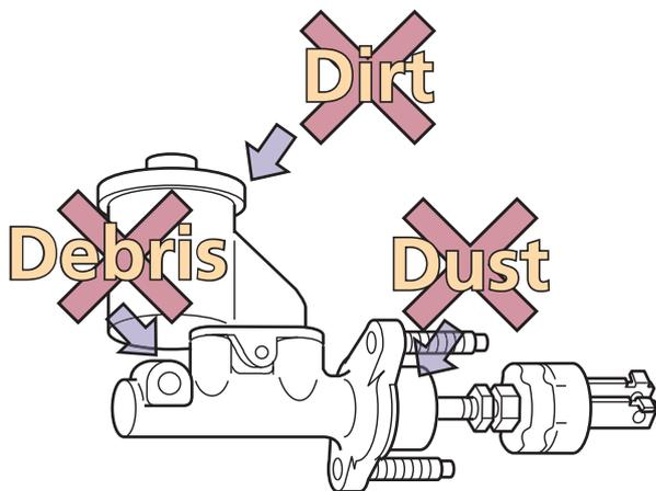
Internal damage may occur, resulting in fluid leakage and improper hydraulic pressure.
