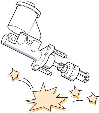
Optimal hydraulic pressure may not be achieved due to damaged internal parts, resulting in incorrect operation and injury.
