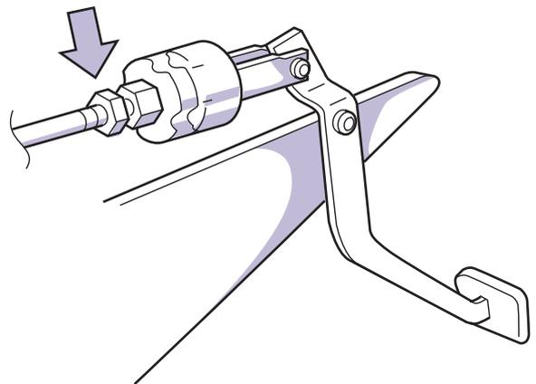
Improper adjustment will cause poor clutch engagement and release.
