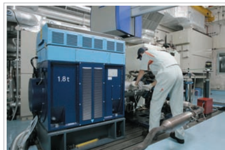
Oil pump test on engine dynamometer
