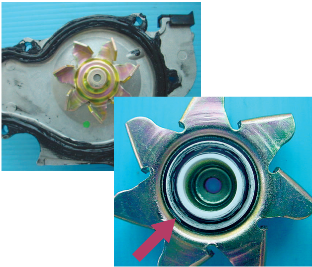
Sealant has interfered with the mechanical seal causing leaks.
