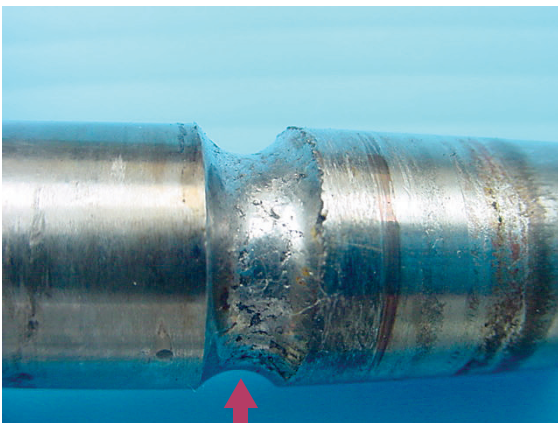
Damage due to overload and seepage
