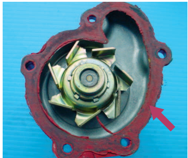
Gasket performance has degraded.
